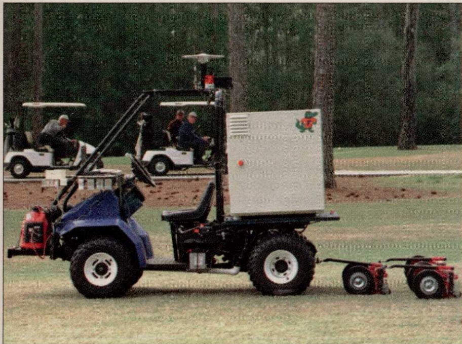
With a fully functional prototype (above), Armstrong's next move is to attract companies like Toro and John Deere to integrate the robotic systems with existing fairway mower models.
