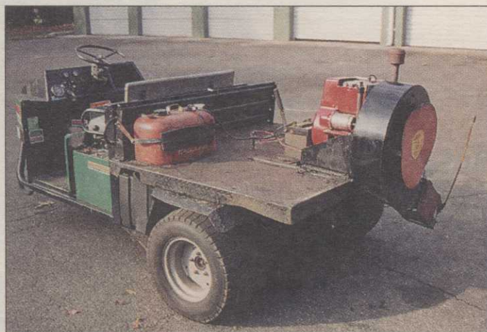
A leaf and debris blower can operate for hours with an auxiliary fuel tank. This version is the one put together for Ridgewood Country Club superintendent Todd W. Raisch by equipment manager Ronny Cestaro.
