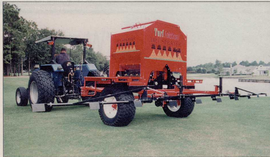
The Dry Sprayer improves seed-soil contact by using air-blast technology to blow seed into the turf canopy.
