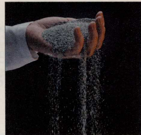
Zinc pellets charge the zinc/air fuel cell.
