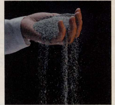
Zinc pellets charge the zinc/air fuel cell.
