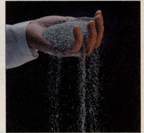
Zinc pellets charge the zinc/air fuel cell.
