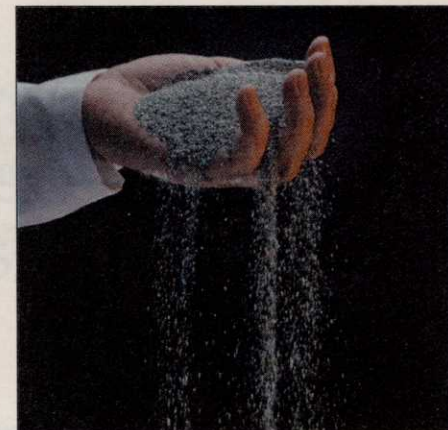
Zinc pellets charge the zinc/air fuel cell.
