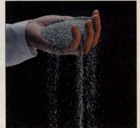
Zinc pellets charge the zinc/air fuel cell.
