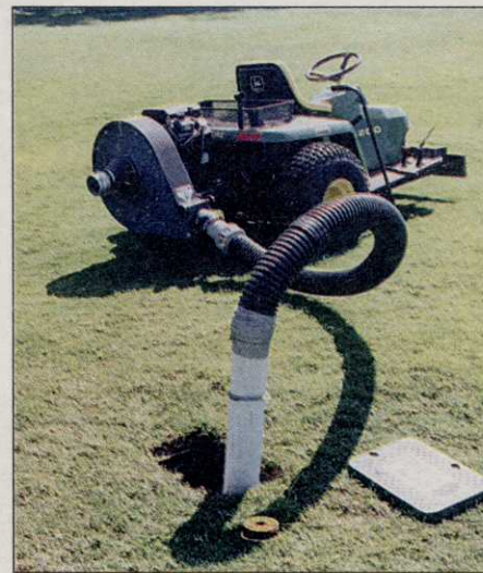
Olde Florida Golf Club demonstrates the effective use of existing equipment with a separate engine-powered blower. The blower can be used elsewhere, such as to blow debris from inside a bunker.
