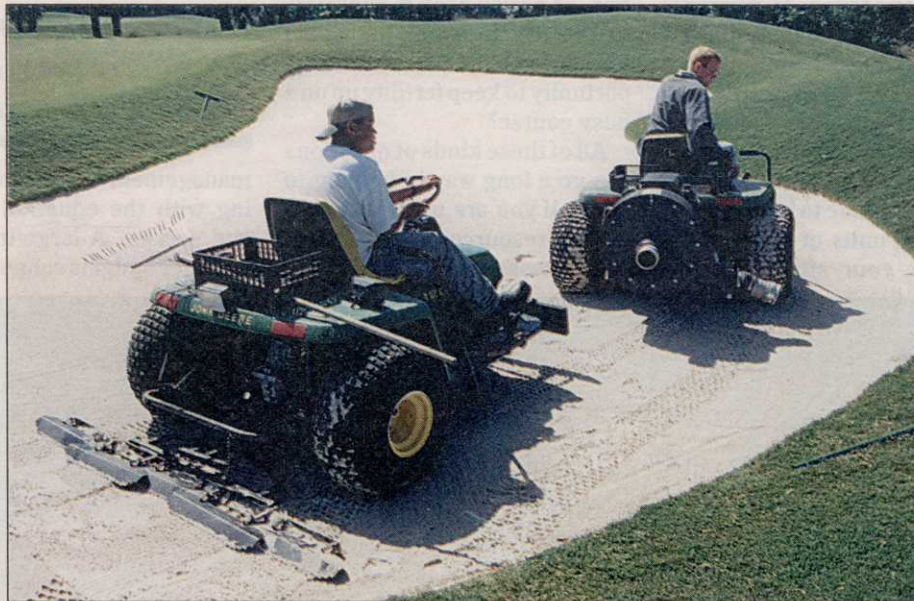
Olde Florida Golf Club demonstrates the effective use of existing equipment with a separate engine-powered blower. The blower can be used elsewhere, such as to blow debris from inside a bunker.
