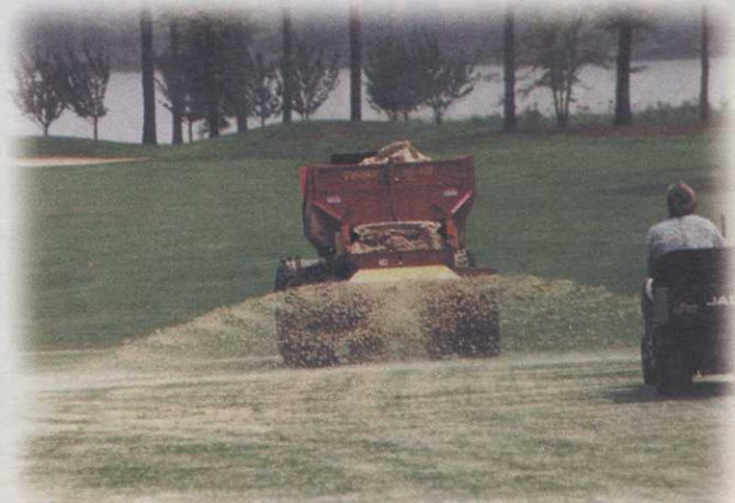
Topdress large areas from 15 to 40 feet wide in minutes using sand, lime, gypsum or compost, without disrupting play.
