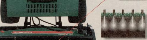
The patented injection process disperses liquids from each nozzle to cover a width of more than four inches beneath the surface. This ensures total target area saturation and eliminates incomplete or inconsistent coverage
