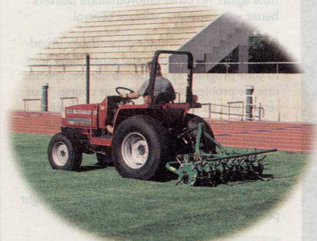
TRACAIRE® —Mount the Tracaire on any tractor with a category "1" 3-point hitch. Cover a 6-foot aerating width with coring, slicing or deep spoon tines.
