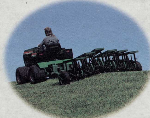
RENOVAIRE® —Designed with the "true contour" principle in mind, each pair of tine wheels is independently mounted to follow the contour of the land.
