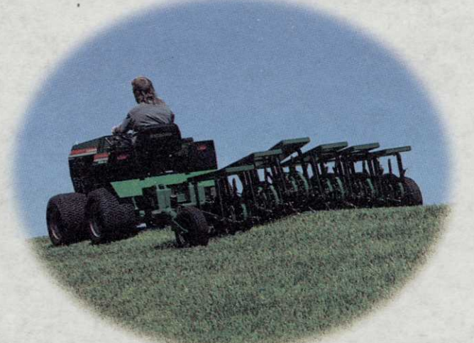
RENOVAIRE® —Designed with the "true contour" principle in mind, each pair of tine wheels is independently mounted to follow the contour of the land.
