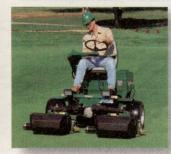
Drive the innovation. Don't worry about cutting into the greens collar. A new automatic center delay compensates for ground speed when raising or lowering the reels so that they all begin and end cutting in the same location on your green.
