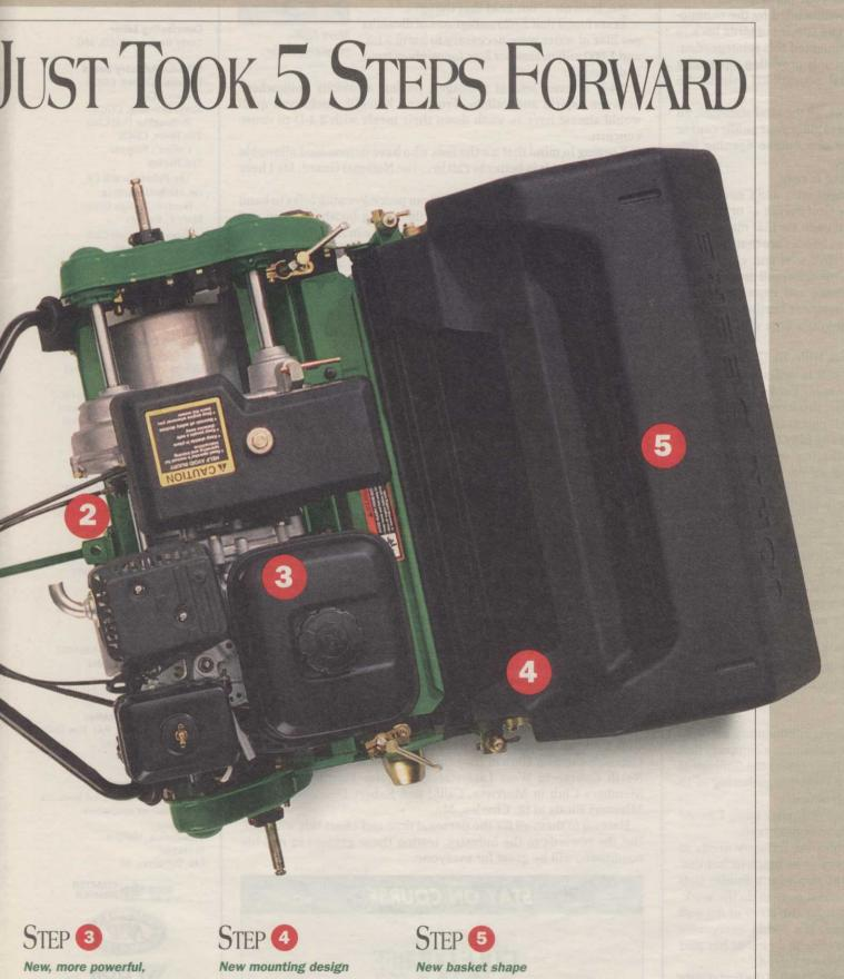
overhead valve engine quietly delivers 4.0 hp. keeps grass catcher more secure.
