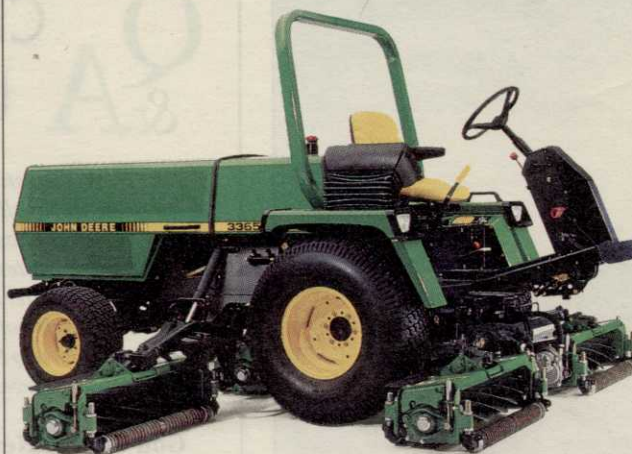
The 3365 Professional Turf Mower delivers a 138-inch cut with five John Deere 30-inch cutting units.
