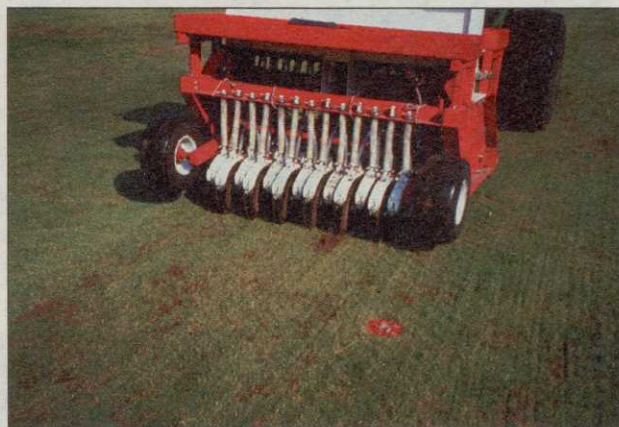
Equipment to apply pesticides below the soil surface has been developed and has shown modest success in enhancing mole cricket control.
