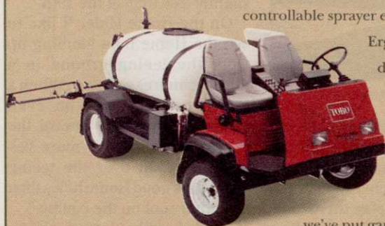
The Multi Pro 5500 features a new drive mechanism for improved climbability and constant speed on varying terrain.
