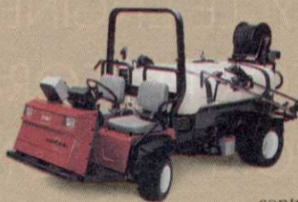
The Workman Turf Spray System combines 200 gallon tank capacity with the mobility of Toro's versatile work vehicle.
