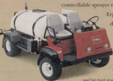
The Multi Pro 5500 features a new drive mechanism for improved climbability and constant speed on varying terrain.
