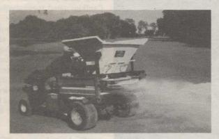
This slide-in top dresser can be used on most turf vehicles. A self contained unit powered by a 5 hp. Briggs & Stratton engine. Can be mounted or removed in minutes. Weight 500 lbs. 18 foot spreading width.
