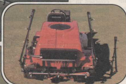
LIGHTWEIGHT AUTOBOOMS FOLD FORWARD FOR SAFE TRANSPORT
