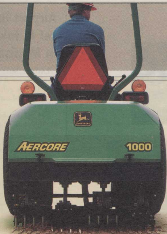
The Aercore 1000 can produce 600,000 holes per hour at a coring swath of 37.5 inches.
