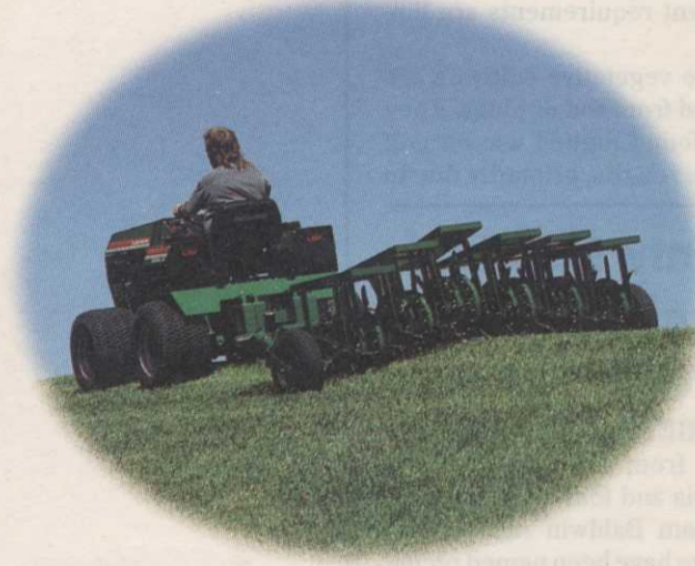
RENOVAIRE® —Designed with the "true contour" principle in mind, each pair of tine wheels is independently mounted to follow the contour of the land.
