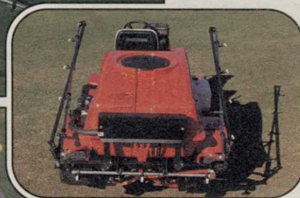
LIGHTWEIGHT AUTOBOOMS FOLD FORWARD FOR SAFE TRANSPORT
