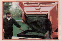
The **MH-400** sits level at 34 inches or can be raised to any height up to 65 inches high—with one simple control lever.
