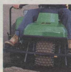
Both front- and mid-mounted implements are now spring-counterbalanced for easier operation.
