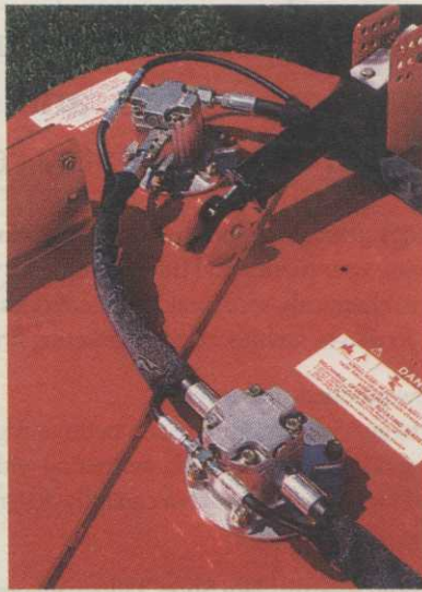
Individual hydraulic motors drive each blade for unmatched cutting power and reduced maintenance.
