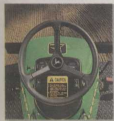
Forty percent less steering effort translates into easier operation for the 1200A.
