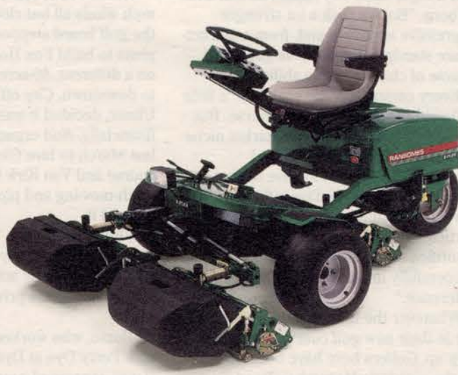
The charge of simple batteries is the fuel for the E-Plex™, the first all-electric triplex greens mower. This technology will change forever the way golf courses are maintained.
