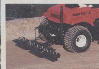
TWIN - PHASE RAKING SYSTEM
