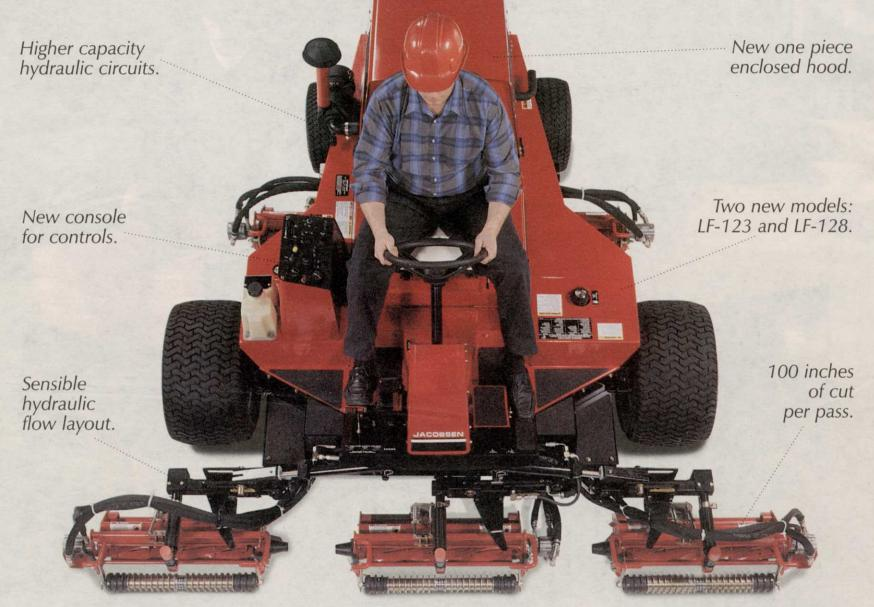
It just makes sense: Start with the top-selling lightweight fairway mower in the world, and introduce two new models. Both the 23-horse LF-123 and the 28-horse LF-128 offer common sense where you need it most.
