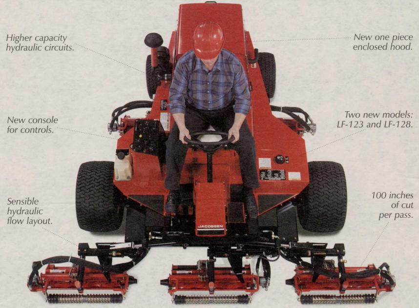
It just makes sense: Start with the top-selling light-weight fairway mower in the world, and introduce two new models. Both the 23-horse LF-123 and the 28-horse LF-128 offer common sense where you need it most.
