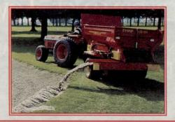
The 3-Way Cross Conveyor attaches to the right or left side and can be attached straight out the back to operate at a 7' extension to the MH-400. The Cross Conveyor will allow you to complete a variety of in house construction or renovation jobs.
