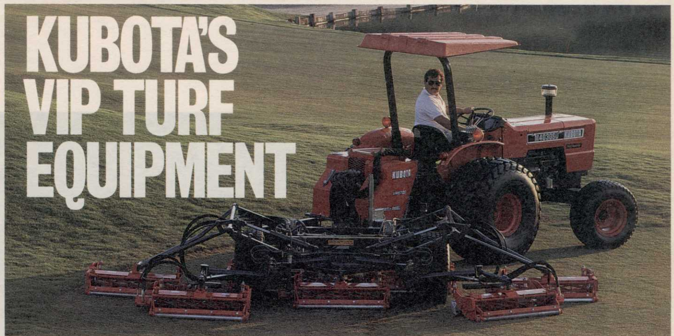
M4030SU with 5-gang Verti-Reel for high production mowing.
