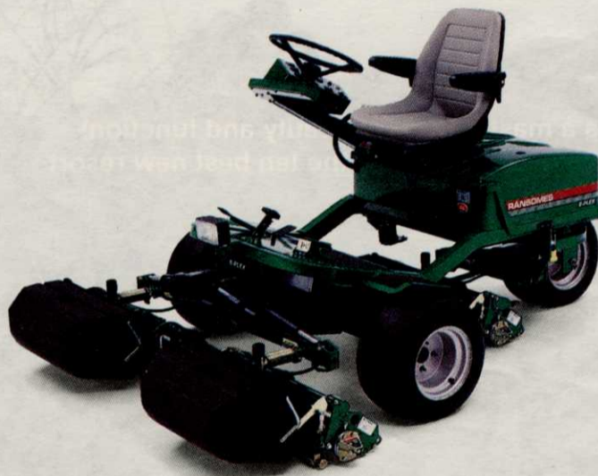
The charge of simple batteries is the fuel for the E-Plex™, the first all-electric triplex greens mower. This technology will change forever the way golf courses are maintained.
