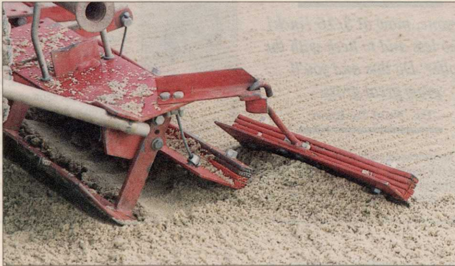
The "Sandpacker" attachments angle (left foreground) can be adjusted by the superintendent to custom-fit his bunker sand maintenance objective.
