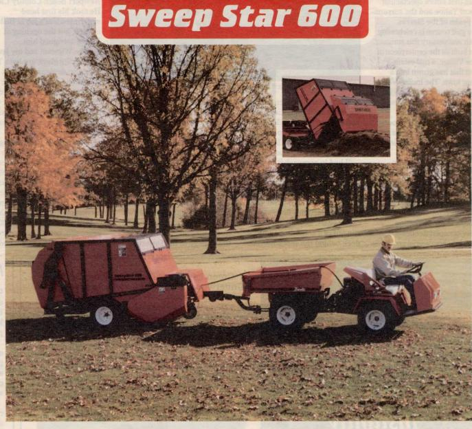
Introducing the Sweep Star 600 – the only pulltype turf sweeper that lets you handle every control function right from the operator's seat, quickly and easily.
