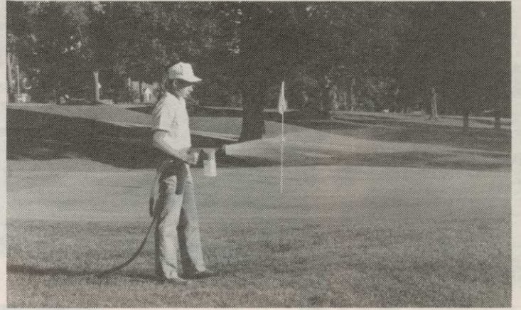
Convenient, cost-effective Pro-Ap delivers consistent, measured quantities of Hydro-Wet RTA—treats 1,000 sq. ft. in less than one minute.
