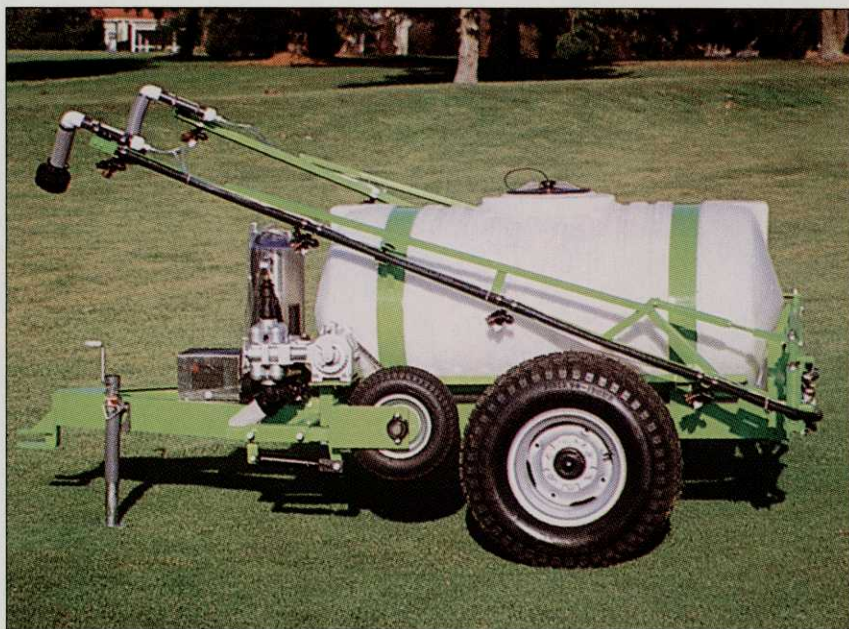
The Turf Runner 300 fairway sprayer, new from Mid-Atlantic Services, features a John Blue Company ground-driven, variable-stroke pump designed to assure accurate spread, completely independent of ground speeds, pressure or tip wear. Standard features include a 300-gallon poly tank, 25-foot hinged truss boom with fore/aft breakaway & auto set, separate full-tank length sparger agitation, and pressure capability up to 120 psi. For more information, call Mid-Atlantic at 1-800-637-0050.
