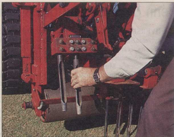
Johnny Burns' block modification, which attaches directly to the Verti-drain, adds major impact to aeration process.
