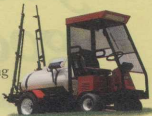
A new optional Pressurized Cab Enclosure prevents entry of pesticide particles.
