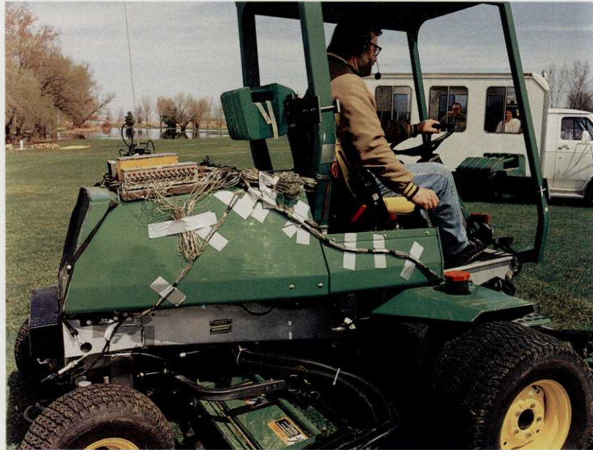
Electronic stress testing monitors and records how well various parts of the machine hold up to the shocks of normal use and abnormal abuse.
