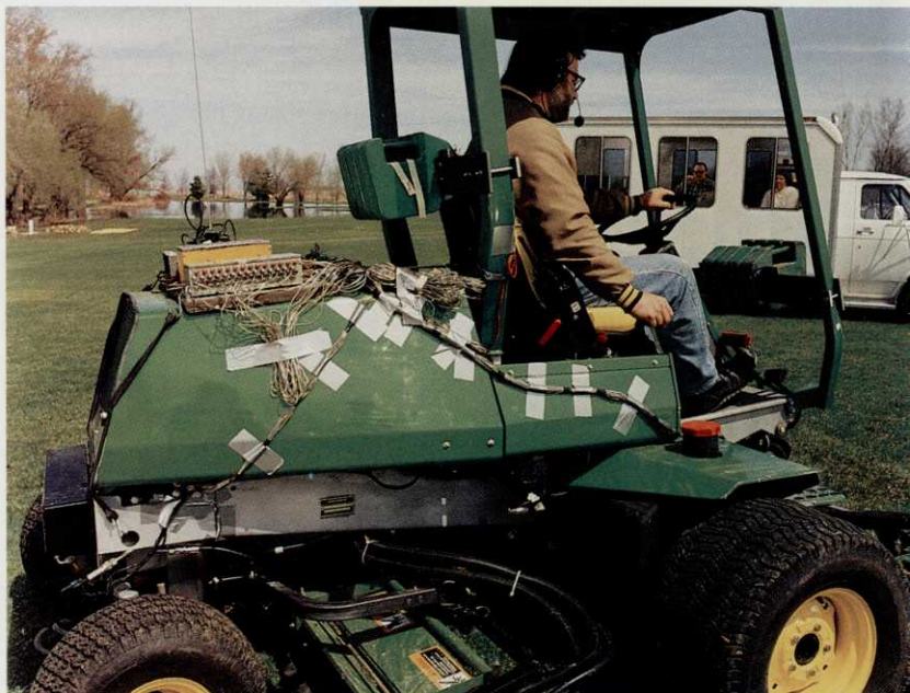
Electronic stress testing monitors and records how well various parts of the machine hold up to the shocks of normal use and abnormal abuse.
