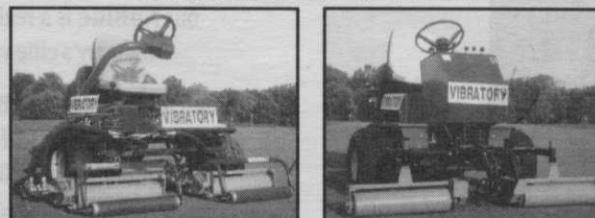
The new TRUE-SURFACE™ vibratory rolling system uses an unbalanced center shaft with an eccentric flyweight to create needed movement of the outer roller, resulting in a smoother & faster putting surface. The "Quick Attach" system allows installation on most riding greens mowers in minutes.
