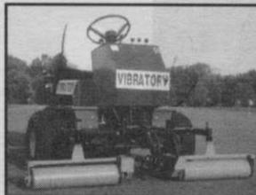
The new TRUE-SURFACE™ vibratory rolling system uses an unbalanced center shaft with an eccentric flyweight to create needed movement of the outer roller, resulting in a smoother & faster putting surface. The "Quick Attach" system allows installation on most riding greens mowers in minutes.
