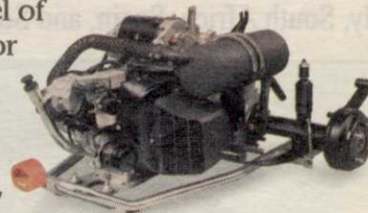
Carryall's Powerful 4-Cycle Gasoline Power Train.
