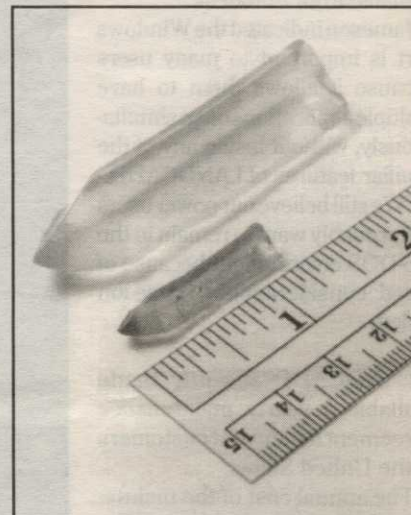
Polymer crystals start out small — but after absorbing several hundred times their weight in water, they grow accordingly.
