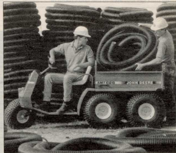
John Deere's 10-horsepower, two-passenger AMT626 runs with a wide stance for stability and versatility.
