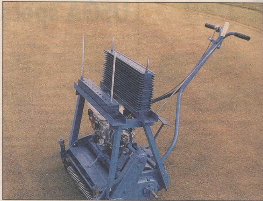
Adding weight to rolling devices is one trick being perfected among superintendents.
