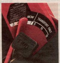
Toro's exclusive variable clip control allows you to calibrate reel speed and mowing speed to give you the highest quality of cut in varying course conditions. Combine that with faster mowing speeds, up to 7.5 mph and 12.5 mph transport speed, and you're going to witness an increase in productivity. All controls are in easy reach of the operator to provide greater comfort.
