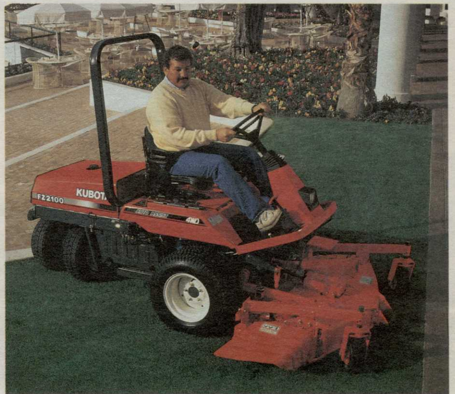
Kubota's FZ2100 with Auto Assist Differential and Zero Diameter Turning Radius.
