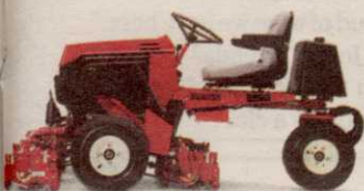
REELMASTER 216 3 wheel drive, gasoline powered 11 blade floating head.
