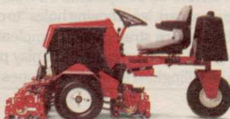
REELMASTER 216-D 2 wheel drive, diesel powered 8 blade floating head.
