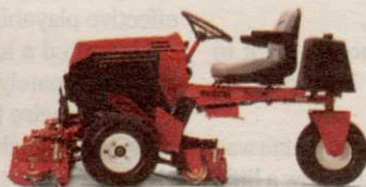
REELMASTER 216 2 wheel drive, gasoline powered 5 blade fixed head.
