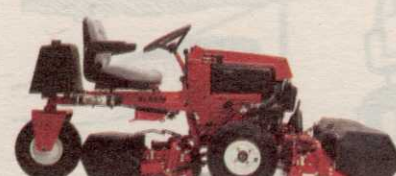
REELMASTER 216 2 wheel drive, gasoline powered 8 blade floating head.
