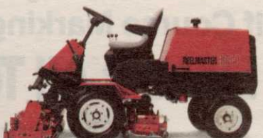
REELMASTER 335-D 2 wheel drive, diesel powered 5 blade floating head.
