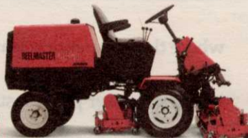
REELMASTER 335-D 2 wheel drive, diesel powered 5 blade fixed head.
