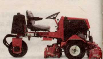
REELMASTER 216-D 3 wheel drive, diesel powered 8 blade floating head.
