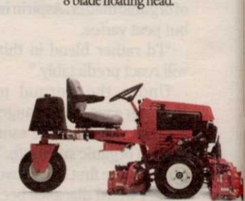
REELMASTER 216 2 wheel drive, gasoline powered 11 blade floating head.
