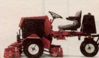
REELMASTER 216-D 3 wheel drive, diesel powered 5 blade fixed head.
